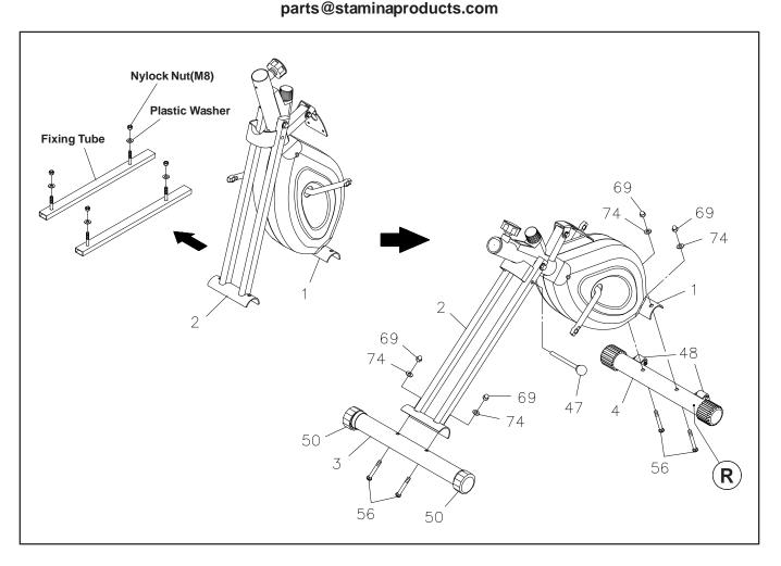
NOTE: Remove the FIXING TUBES, WASHERS, and NUTS from MAIN FRAME(1) and REAR FRAME(2) before any assembly. These parts are only for packing, do not dispose of the packing materials until assembly is completed.
